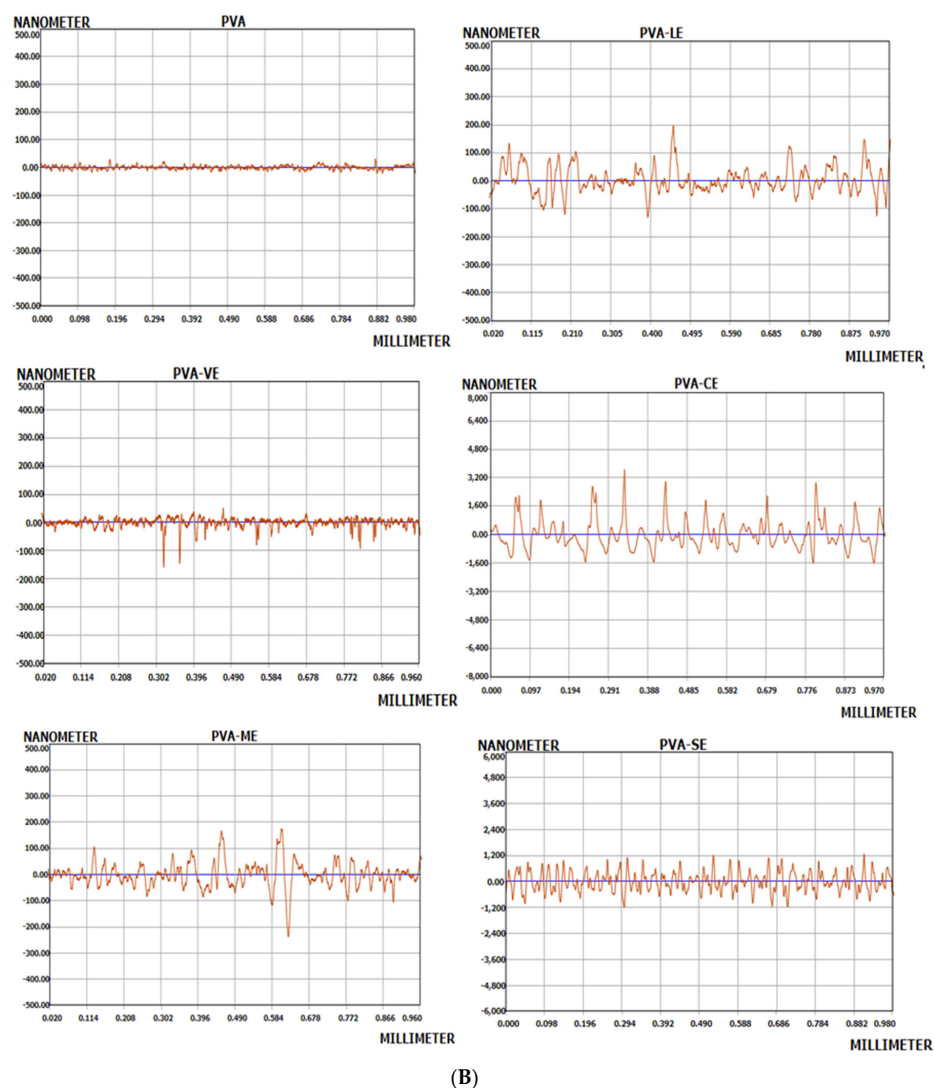
Figure 5. (A) Surface morphology analysis with Raman confocal microscope images PVA (a); PVA-VE (b); PVA-ME (c); PVA-LE (d); PVA-CE (e); PVA-SE (f) and (B) Profiler roughness measurements.
