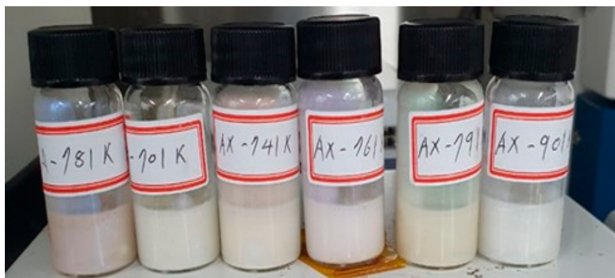
Figure S1. Color solutions composed of pearlescent pigments and optical adhesives (NOA) matrix. From left, A-781K (Splendor Blue), AX-701K (Dazzling Gold), AX-741 (Dazzling Red), AX-761 (Dazzling Violet), AX-791K (Dazzling Green) and AX-901K (Dazzling Standard)
