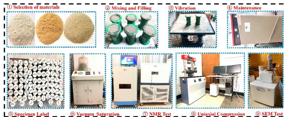
Figure 1. Specimen making and testing.
