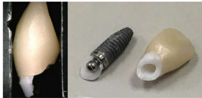
Figure 6. Typical fracture mode in All-Zr group (oblique fracture line starting from the buccal aspect in the internal hexagon region).
