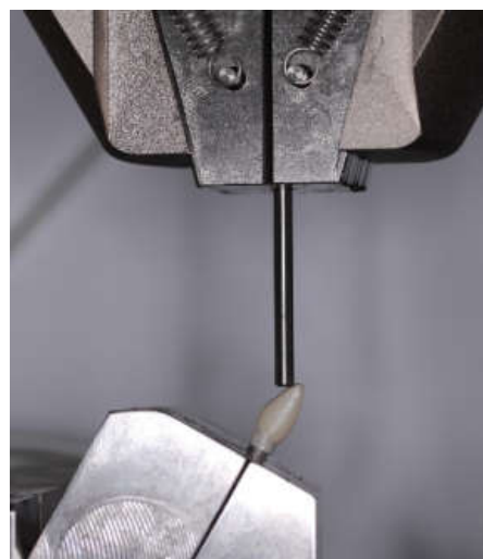
Figure 4. Loading of the assembled specimen with a universal testing machine at 30°.
