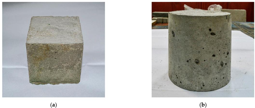
**Figure 3.** Concrete samples: (a) cubes; (b) cylinders.
