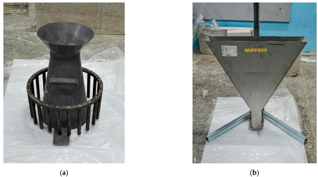
**Figure 2.** Devices for monitoring the rheological characteristics of SCC mixtures: (a) a cone for determining mobility; (b) V-shaped flow funnel.
