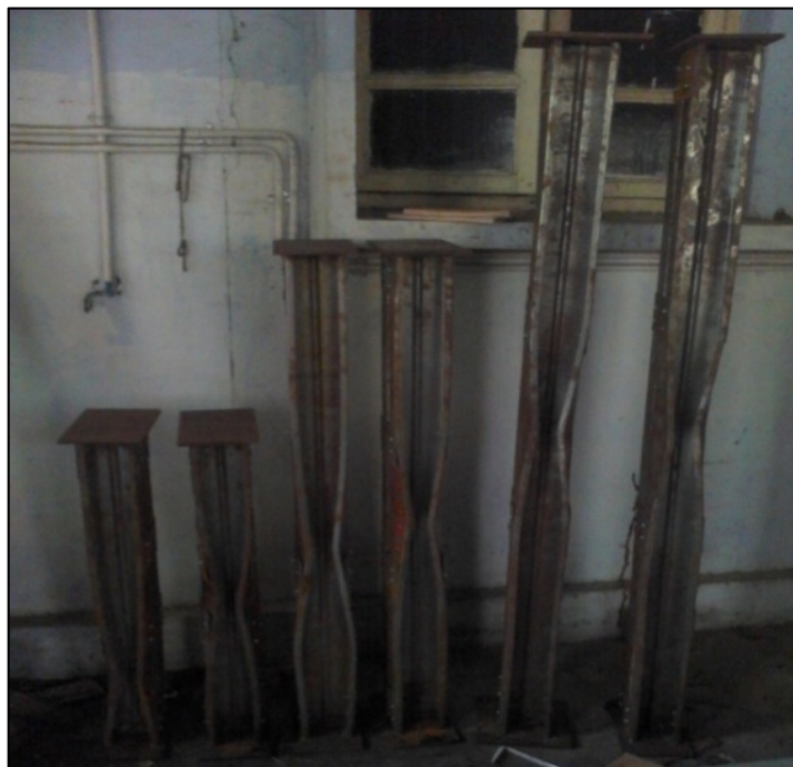
Figure 7. Some of the buckled specimens after load subsection.
