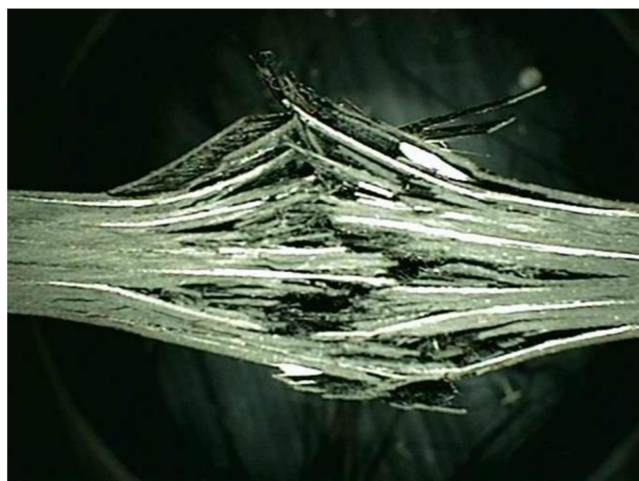
Figure 4. Investigation of the fracture surface of the compression specimen.
