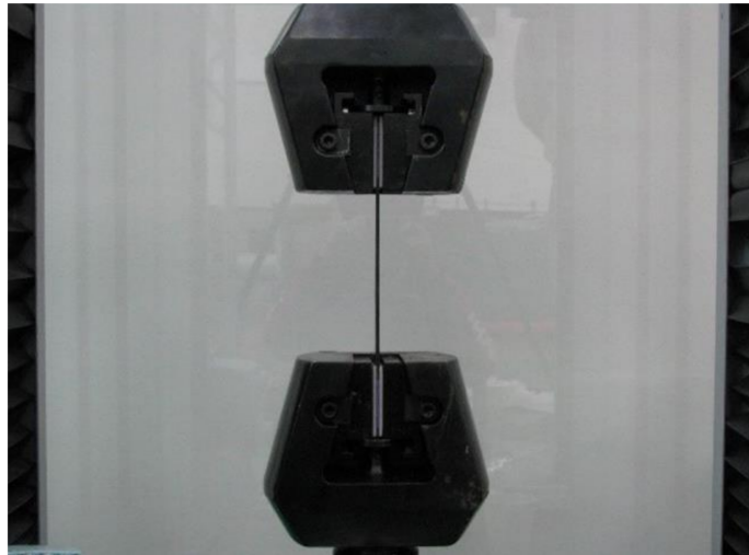
Figure 1. Tensile test of the manufactured specimen.
