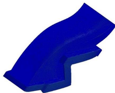
Figure 7. Finite element model of S-duct.
