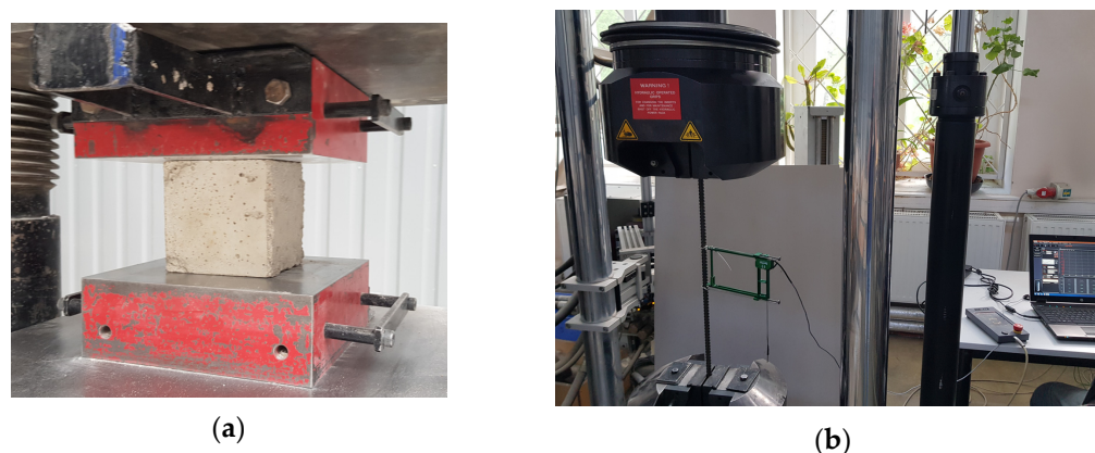
Figure 5. Determination of technical characteristics of the concrete and reinforcements. (a) Determination of the compressive strength of concrete cubes, (b) tensile strength of reinforcements.
