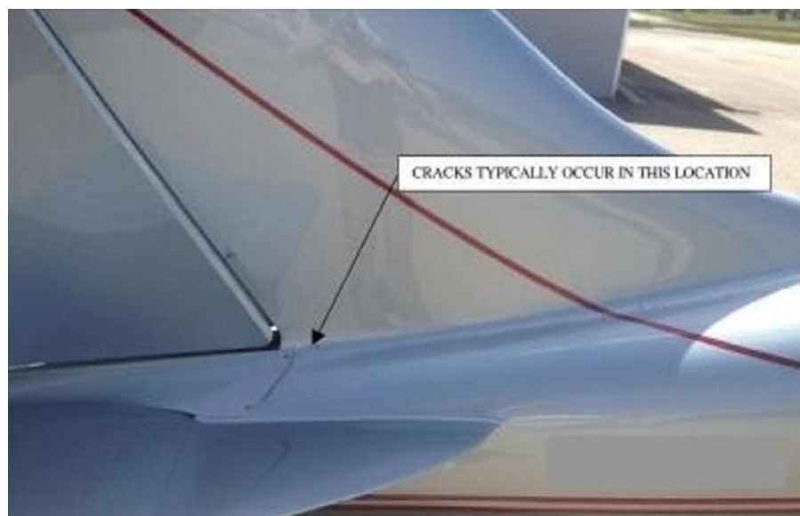
Figure 1. Crack in aircraft body [3]. Reprinted under the Creative Commons (CC) License (CC BY 4.0).
