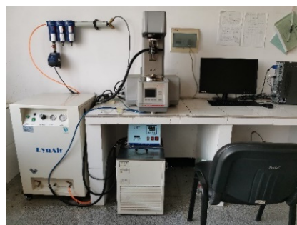
Figure 2. Anton Paar MCR 102 rheometer.
