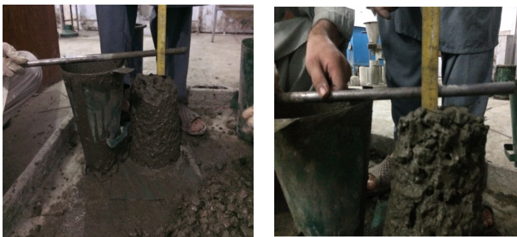
Figure 6. Slump cone test of fresh concrete.
