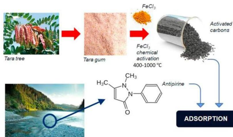
**Figure 13.** Preparation process of Tara gum-derived activated carbon and its application for adsorption antipyrine in water [242].
