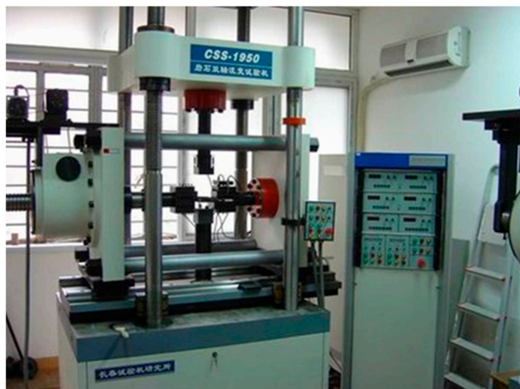
Figure 4. Biaxial rheological testing system (CSS-1950).
