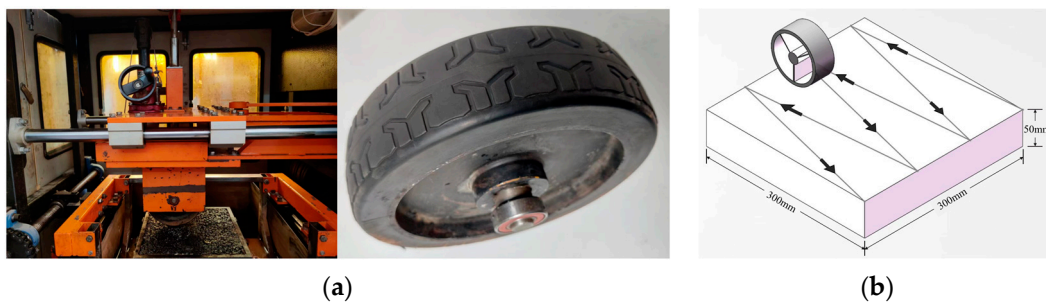
Figure 2. Accelerated pavement test: (a) kneading machine and tire and (b) tire kneading path.
