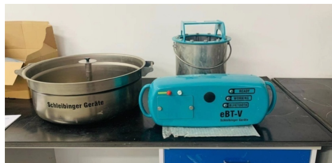
Figure 4. eBT-V concrete rheometer.
