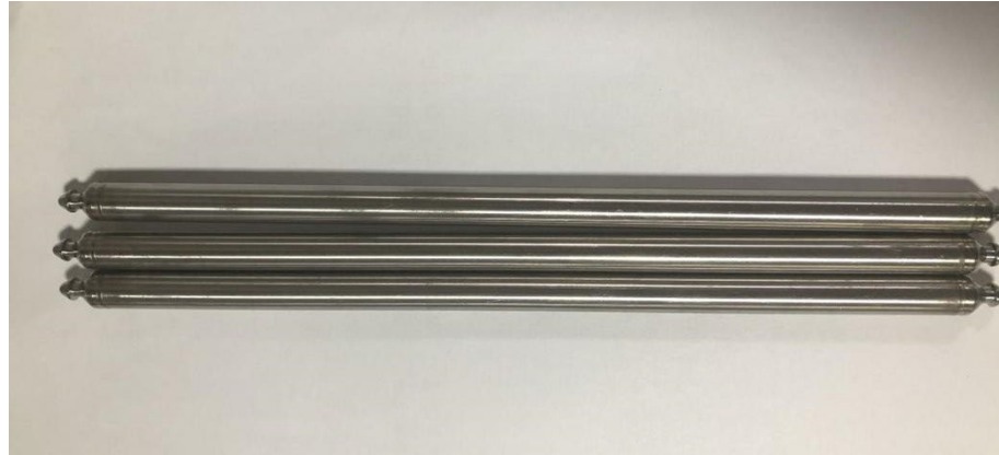
Figure 1. Zr–Sn–Nb alloy single-sided tube samples.
