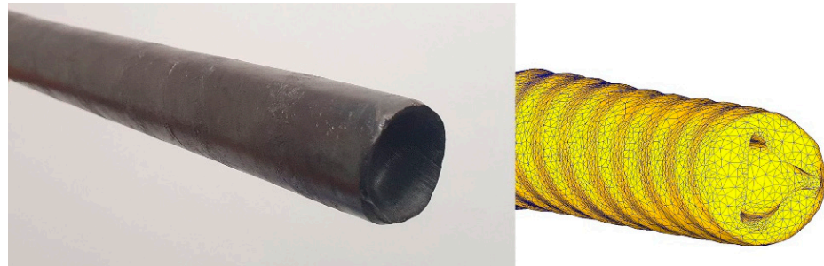
Figure 8. Comparison of the shape change of the rolled experimental bar with the previously obtained FEM model.
