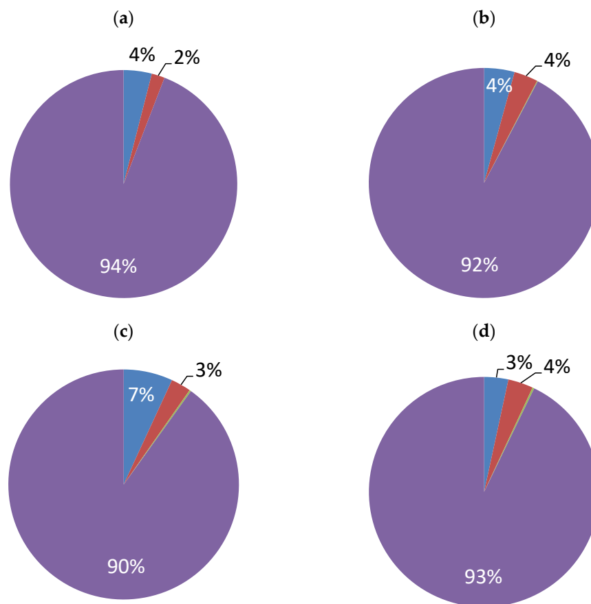
Figure 4. Atomic composition (%) (■—C, ■—O, ■—Ni) of the coatings obtained from (a) bath I (without additives), (b) bath II (15 mM of saccharin), (c) bath III (6 mM of [\text{H}_2\text{EDTA}^{2+}][\text{HSO}_4^-]_2 ), and (d) bath IV (15 mM of saccharin and 6 mM of [\text{H}_2\text{EDTA}^{2+}][\text{HSO}_4^-]_2 ).
