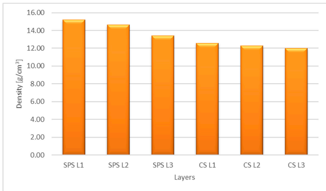
Figure 8. The layers densities after SPS and CS.
