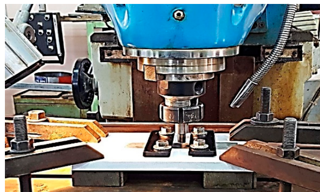
Figure 4. The FSSW process.
