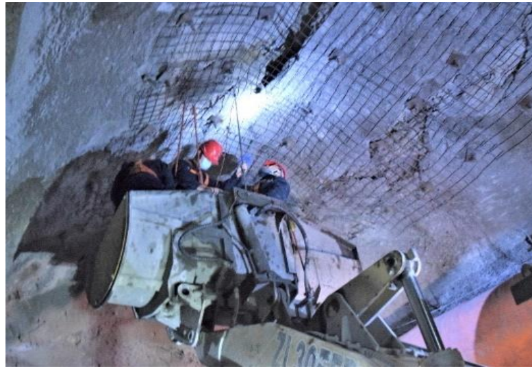
Figure 6. Borehole image monitoring of the surrounding rock of the horsehead roadway.
