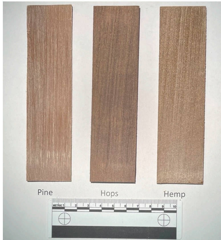
Figure 7. Photograph of the pine-, hemp- and hop-extruded WPCs.
