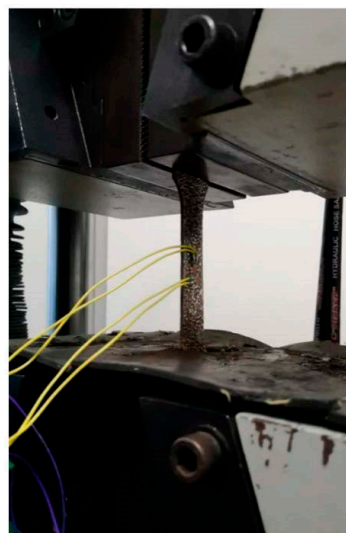
Figure 4. Steel coupon tensile test after sulfate corrosion layout of strain gauges.
