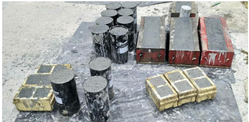
Figure 24. Typical samples cast for different mechanical properties.
