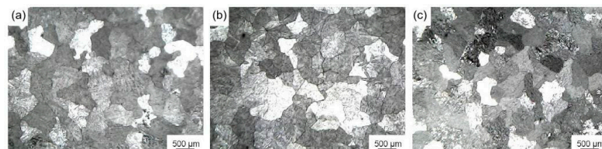
Figure 11. Microstructure of pure aluminum after being refined by Al-Ti-C grain refiners with various extrusion ratios (add 1 wt.%): (a) extrusion ratio 13 grain refiner (4#), (b) extrusion ratio 20 grain refiner (5#), (c) extrusion ratio 30 grain refiner (6#).
