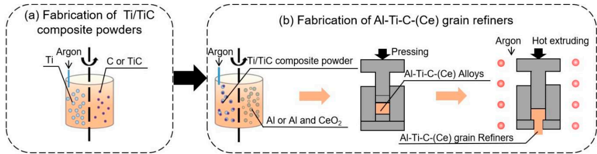
Figure 1. Flow diagram for the preparation of Ti/TiC composite powder and Al-Ti-C-(Ce) grain refiners: (a) fabrication of ball milling loaded and in-situ reaction Ti/TiC composite powder, (b) fabrication of Al-Ti-C-(Ce) grain refiners.
