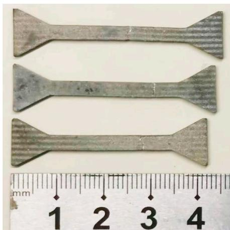
**Figure 7.** The 450T6 specimens with a 48% DP-region fraction tensile-tested until failure at different temperatures.
