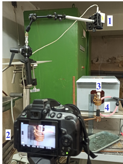
Figure 1. The station used to measure the position and temperature of the batch.
