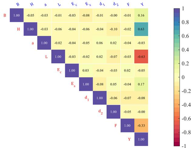
Figure 3. PCC between the variables of a RC simply supported beam.
