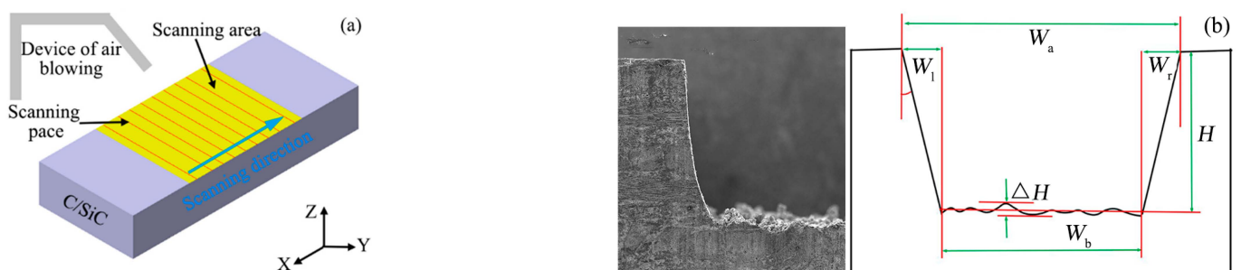
Figure 3. Schematic diagram of groove scanning trajectory and evaluation characteristics of grooves. (a) Schematic diagram of groove scanning trajectory. (b) Evaluation characteristics of grooves.
