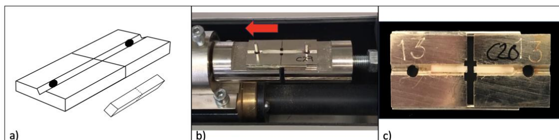
Figure 6. Microtensile test. (a) Schematic representation of a plate and a beam. (b) LMT100® machine before test. (c) Broken beam.
