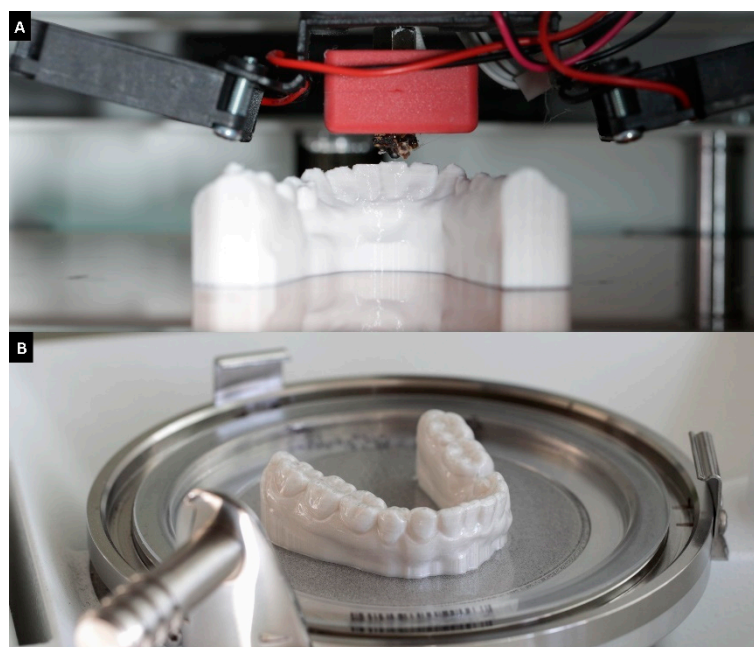
Figure 2. Printed FFF model on printing plate (A), model with thermoforming foil (B).
