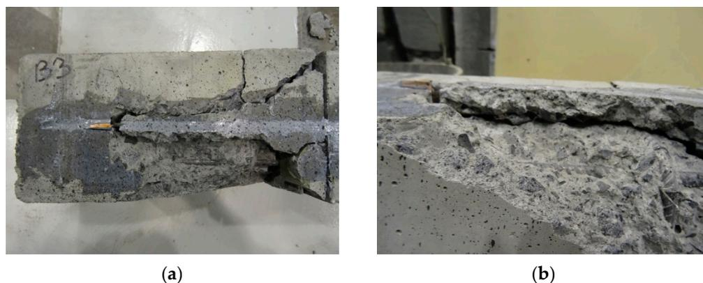
**Figure 5.** RC element failure: (a) underside of series 2 element; (b) partial sliding out of the strip from the copper flat bar clip, together with its debonding from the concrete cover (underside of the reinforced element).
