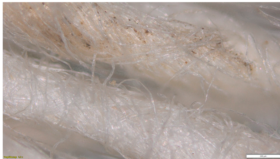
Figure 5. Microscope image of the uncoated yarn sample, showing the damaged fibers (magnification \times 2.5 ).
