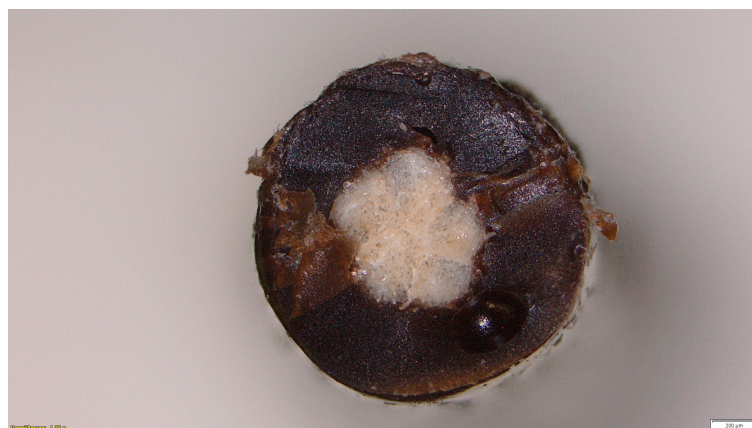
Figure 3. Microscopic image of yarn cross-section of coated sample 1 (magnification \times 1.25 ; diameter of coated yarn approx. 946 \mu\text{m} ).
