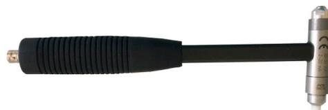
**Figure 10.** Modal hammer PCB model 086C03 used for testing.
