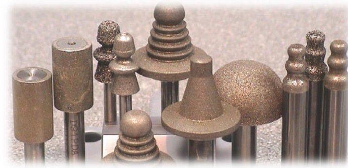
Figure 22. Pin grinding wheels with single layer diamond coating [76].
