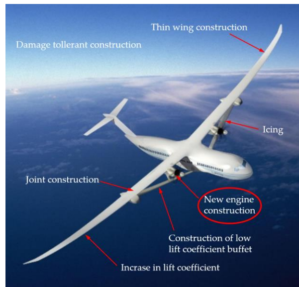
Figure 3. The Transonic truss-braced wing (TTBW) concept and the selected development challenges of the project.
