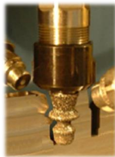
Figure 29. Pin-grinding wheel with cBN coating and visible nozzles supplying the electrolyte to the machining zone [37]. “Reprinted/adapted with permission from Ref. [37]. 2014, Elsevier”.
