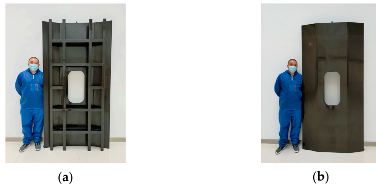
Figure 7. Composite longitudinally and transversely stiffened panel by HRTM: (a) stiffening surface; and (b) skin surface.
