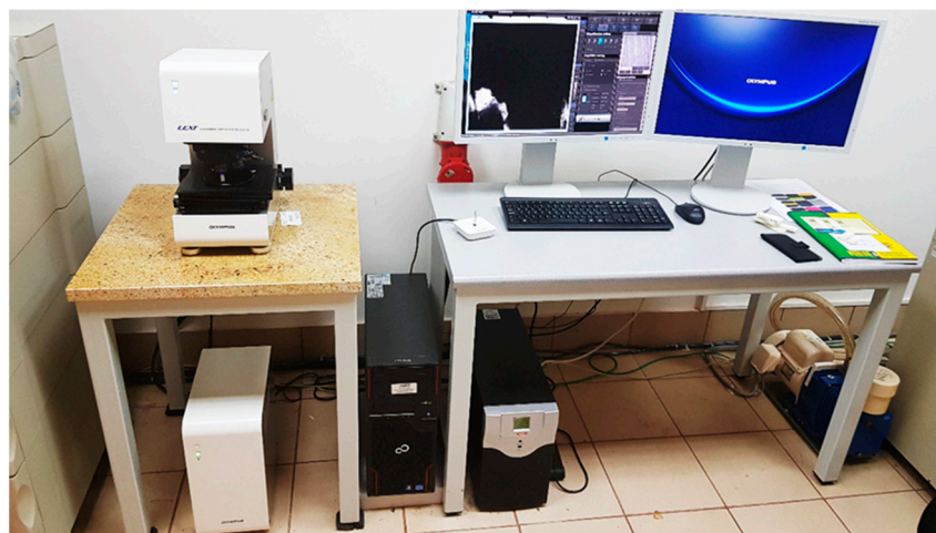
Figure 5. Olympus 4100 LEXT confocal microscope used in the research.
