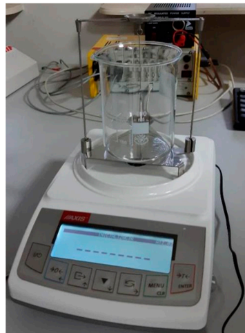
Figure 3. The measurement setup for the density measurement of the samples is shown in Figure 1.
