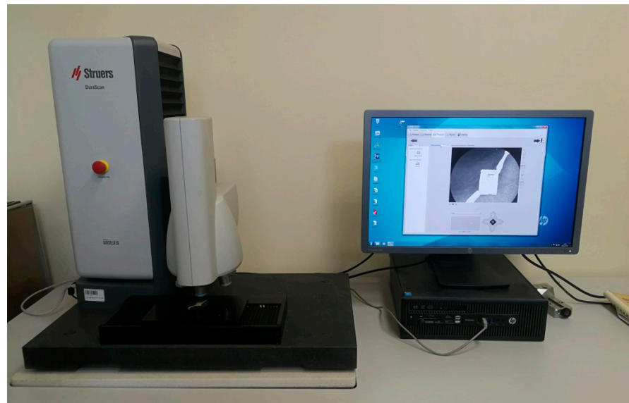
Figure 6. Struers DuraScan 70 hardness tester used in the research.
