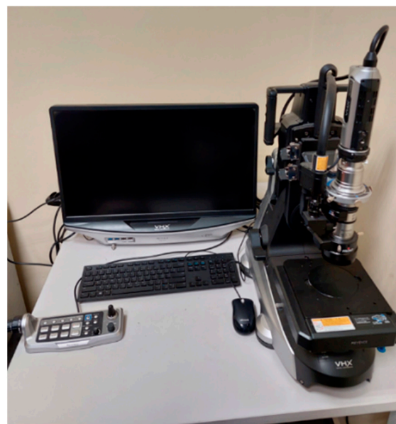
Figure 7. Keyence VHX7000 digital microscope used in the research.
