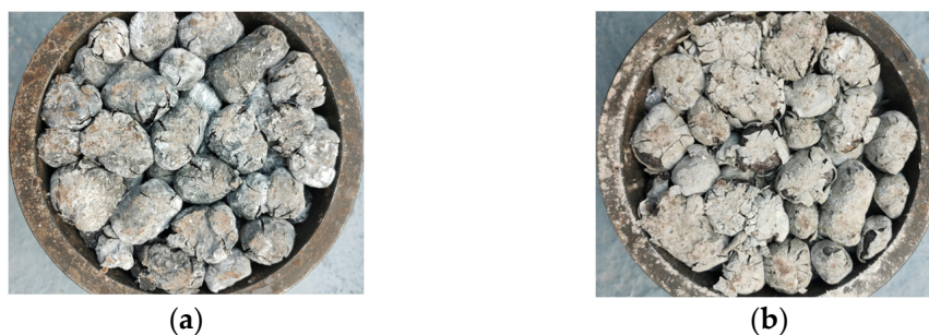
Figure 13. The failure mode of the PCA after cylindrical compress strength test. (a) Epoxy resin-encapsulated PCA; (b) Superfine cement-encapsulated PCA.
