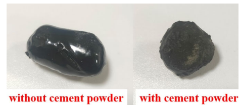
Figure 6. Physical image of epoxy resin PCA before and after wrapping with cement powder.
