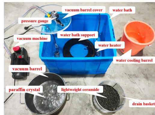
Figure 7. Self-made phase change aggregate preparation equipment.
