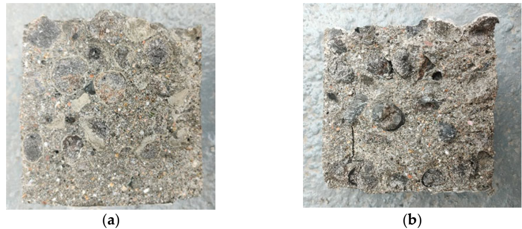
Figure 23. Fracture section of concrete after splitting tensile test. (a) Unencapsulated concrete; (b) Encapsulated concrete.
