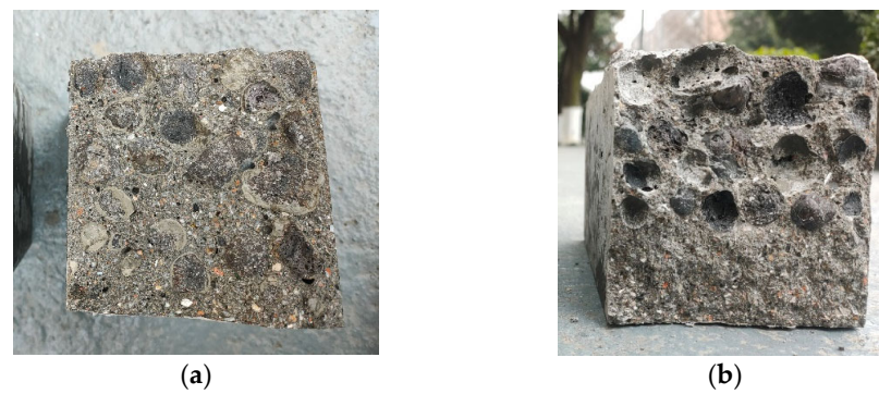
Figure 21. Fracture section of concrete after flexural test. (a) Unencapsulated concrete; (b) Encapsulated concrete.
