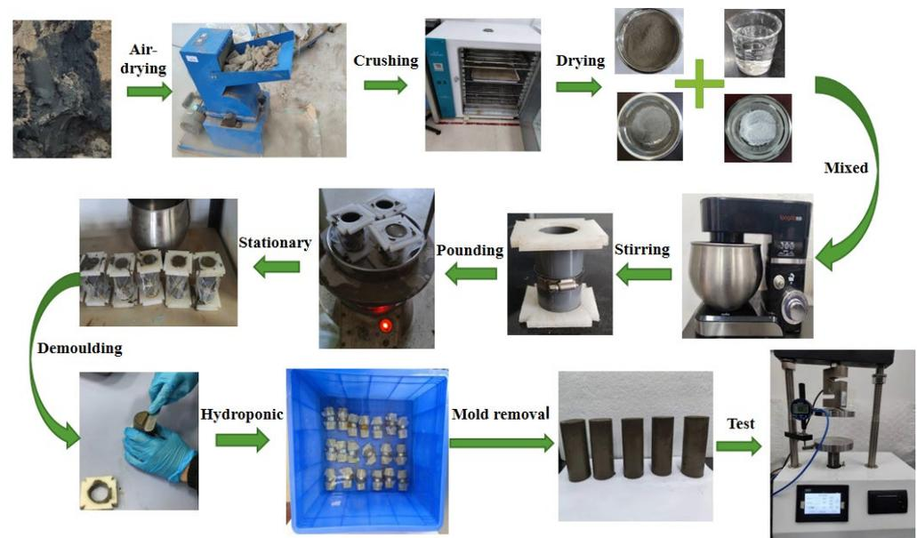
**Figure 3.** Preparation process of modified soil specimens.
