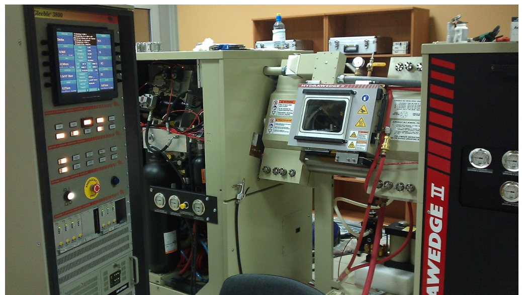
Figure 2. The Gleeble 3800 plastometer testing equipment.
