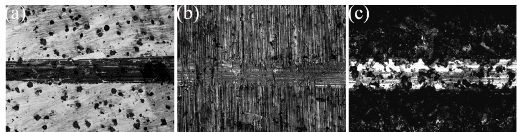
Figure 16. Wear traces under laser confocal observation. (a) Substrate surface; (b) laser-remelted surface; (c) prefabricated laser-melted surface.
