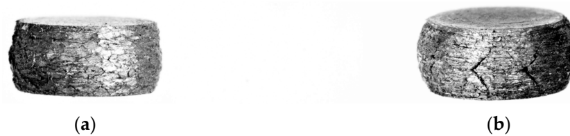
Figure 10. Exemplary photos of composite samples after compression of aluminum matrix composites with the addition of (a) 2.5 wt.% of SiC and (b) 7.5 wt.% of SiC.
