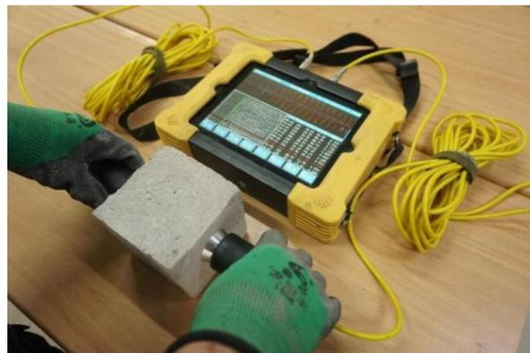
**Figure 4.** Ultrasonic wave velocity test of AASR foamed concrete.
