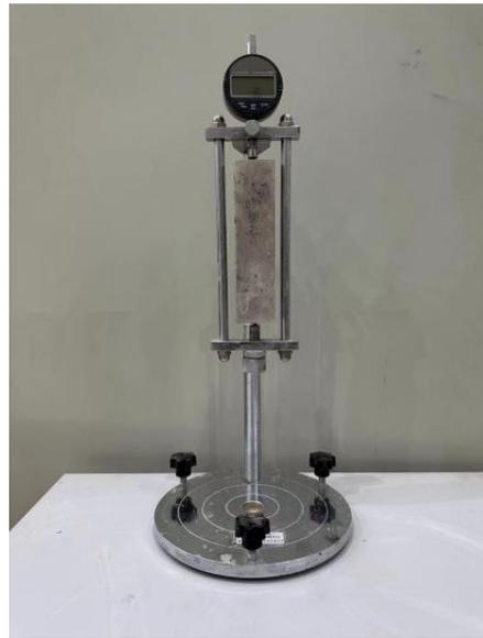
**Figure 3.** Drying shrinkage test of AASR foamed concrete.
