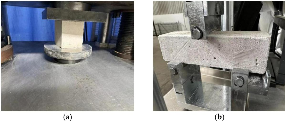
**Figure 1.** Measurement of mechanical properties of AASR foamed concrete, (a) Compressive strength test; (b) Flexural strength test.
