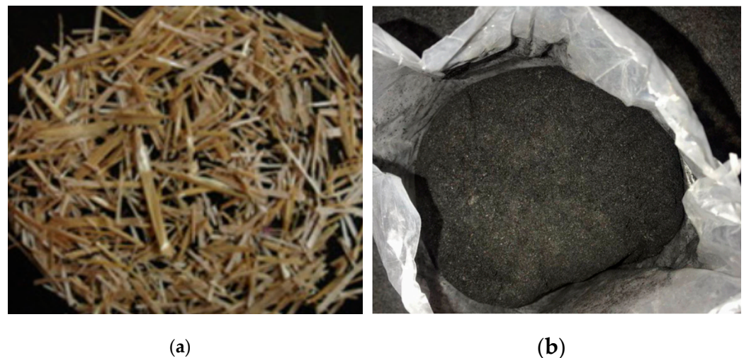
Figure 20. The appearance of wheat stalk and WSA [170,171]. (a) Wheat stalk. (b) WSA.
