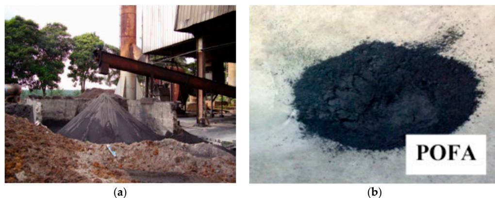
Figure 4. Production of POFA [62,63]. (a) Biomass factory. (b) Palm oil fuel ash.
