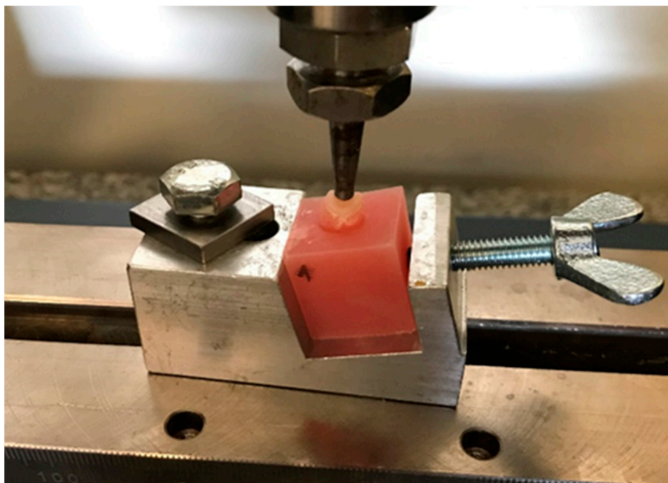
Figure 2. Sample placed in a universal testing machine.
