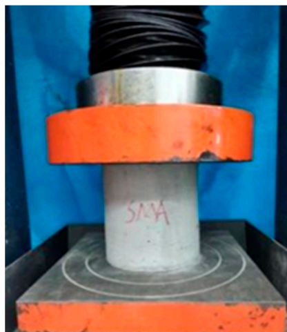
Figure 2. Compression test of hollow cylinder.
