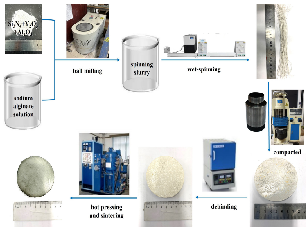
Figure 1. Schematic diagram of Si 3 N 4 /BN fibrous monolithic ceramic preparation.
