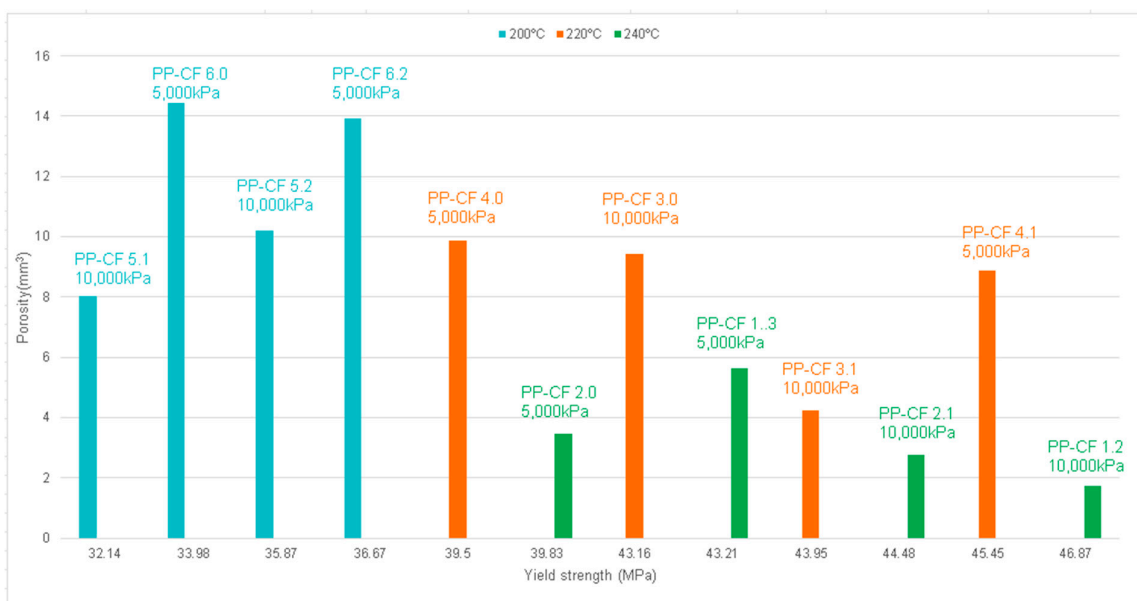
Figure 21. Porosity versus yield strength for carbon-fiber-reinforced polypropylene.
