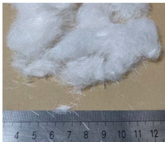
Figure 4. Photograph showing the discrete polypropylene fibers.
