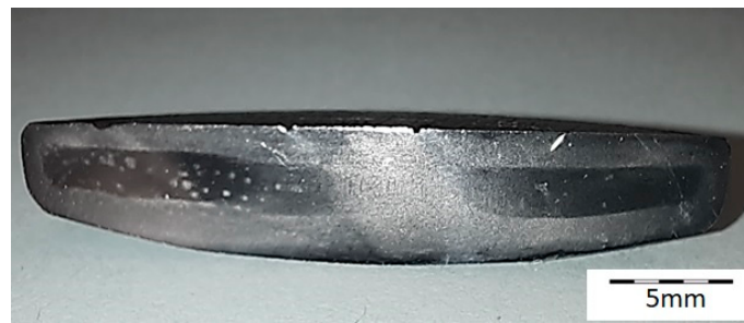
Figure 13. Visible two zones in the cross section made on the valve head. Plane B-B'. Stereoscopic microscopy images, etching with aqua regia ( \text{HNO}_3 + 3\text{HCl} ).
